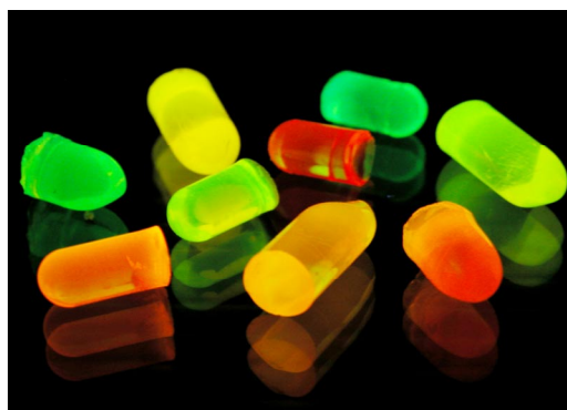
Figure 2. Ionic liquid-based polymer-CdTe NCs composites.
